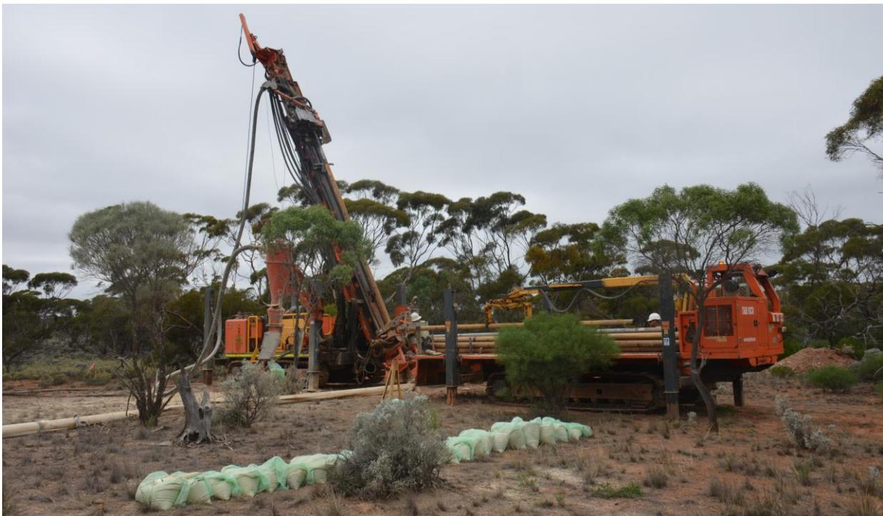
Figure 1: GMP drilling the first of three RC pre-collars for diamond drillholes on EL 5949
