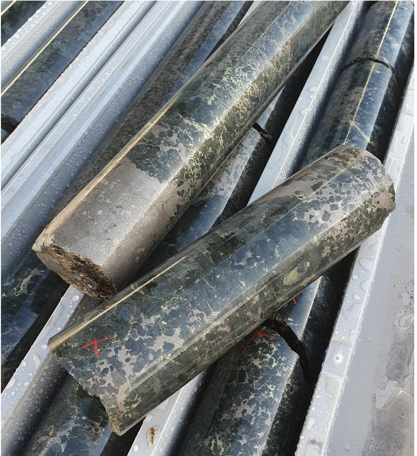
Figure 4. JD006 specimen from ~35m down-hole (new G3 Zone) – coarse grained sulphides (pyrrhotite-chalcopyrite-pentlandite) in pegmatoidal pyroxenite.
